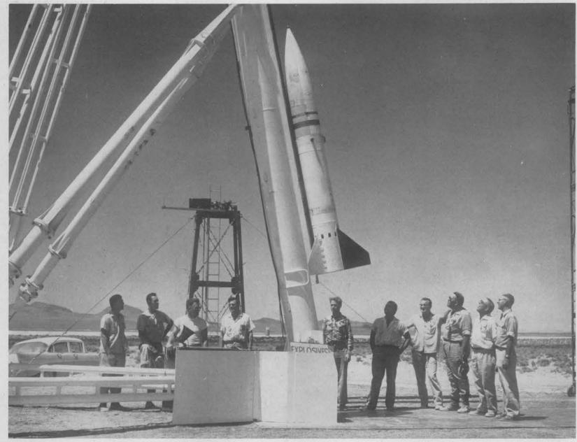
SINGLE-STAGE ROCKET launched last month by Sandia Corporation at the Tonopah (Nevada) Ballistic Range is shown here in the first photo to be released of the operation. The 12-foot rocket attained an altitude of 80,000 feet. Inspecting the rocket before
